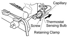
Figure 32 - Removing Thermostat Sensing Bulb
